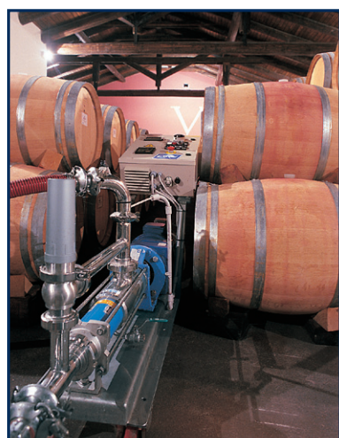
MAE series with electrical control panel for remote On/Off control from the stainless steel suction probes
